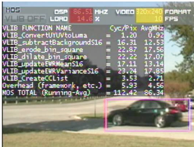
Fig. 5: Screen shot of MOS implementation running on the DM6437 with unoptimized library. The loading on the DSP is approximately 86 MHz for processing a 320x240 pixel video sequence at 10 frames per second.
